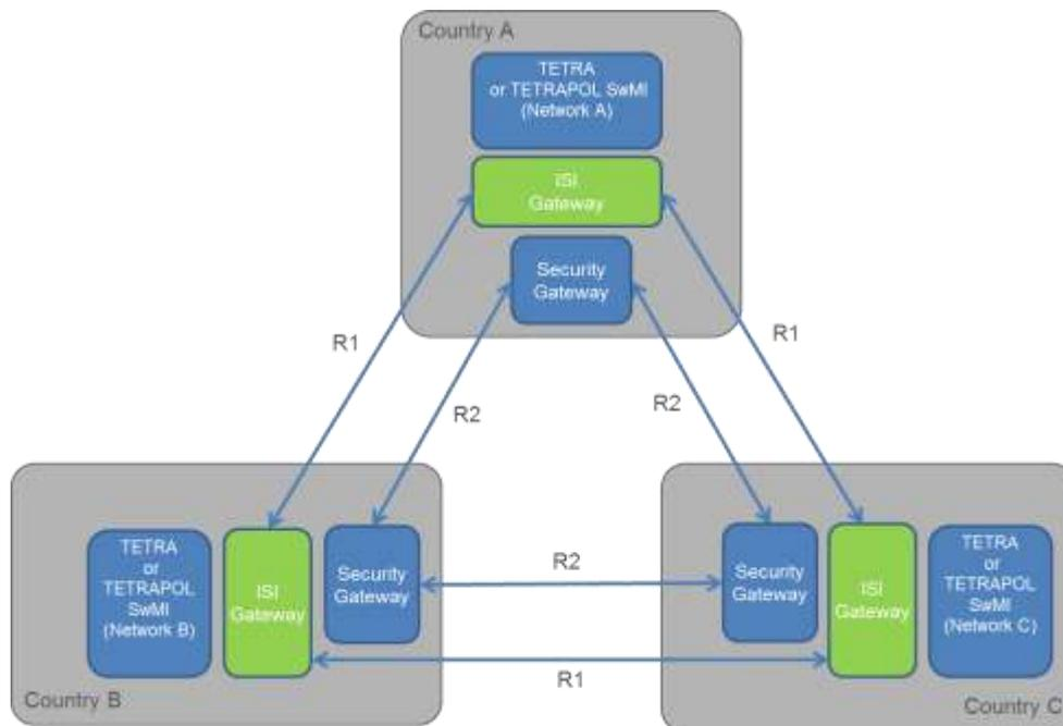
**Figure 7.** Interconnection configuration with three PPDR networks
