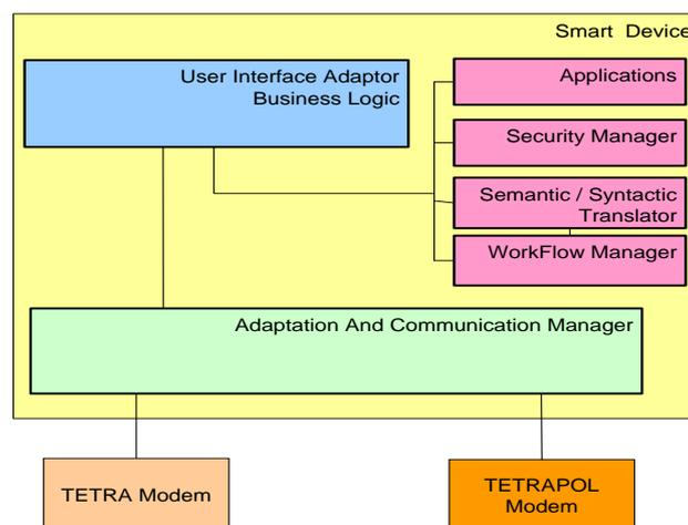
**Figure 10.** Proposed terminal architecture
