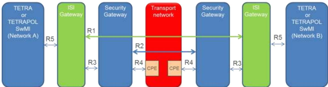
**Figure 5.** Architecture reference model of the ISI cloud network
