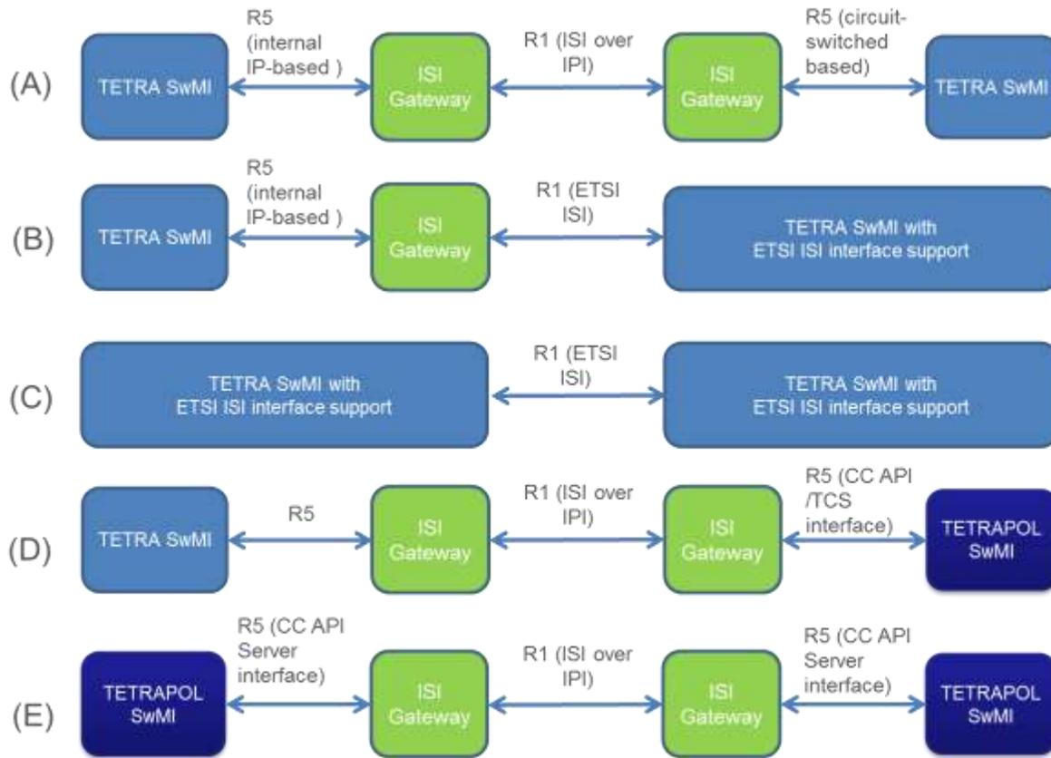
**Figure 6.** Interconnection configurations based on the different possible implementations of R1 and R5 interfaces
