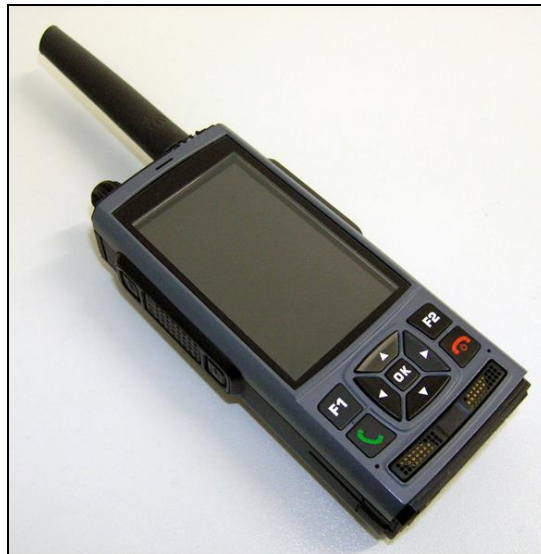
Figure 2 FNM TETRA radio with embedded Android device.
