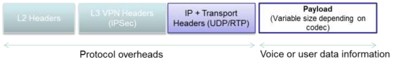
Figure 4. ISI voice and data traffic encapsulated in the payload of IP packets
